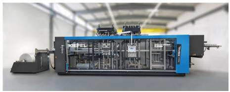
Live demonstration: The SPEEDFORMER KMD 78 Smart from Kiefel offers maximum output and efficiency and is used for the manufacturing of food and non-food plastics packaging using various materials. © KIEFEL GmbH
