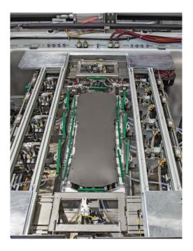
Figure: Tailored-Blank precision cut blank in the new Tailored-Blank-3D servo gripper frame.
