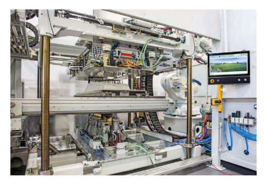
Figure: Laminating station of the TBL vacuum lamination system.
