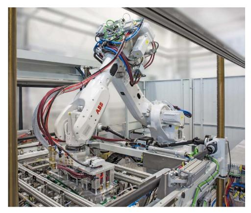
Figure: Forming station with robots for lamination process and parts handling of the vacuum lamination system.
